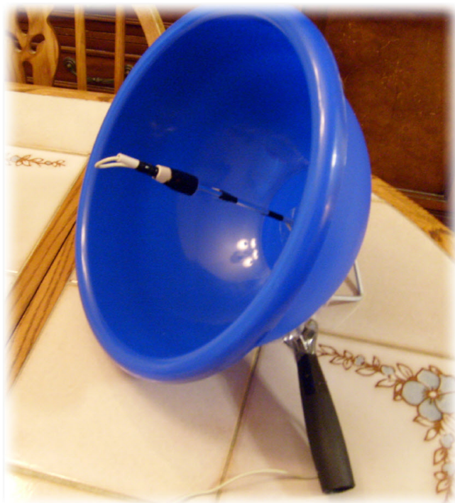
A homemade parabolic microphone. It provides improved reception of distant bugs!
